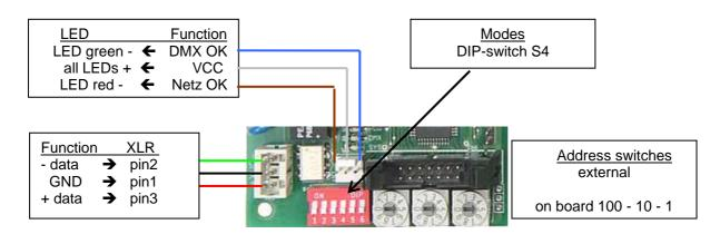
The DMX connector is an cage-clamp type, to open a clamp you should use a 2.5mm flat screw driver. To fix the clamp in the open state put the screwdriver in the square hole near the round hole the wire has to put in.
