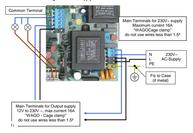
The drawing shows a typical application for 230V~ Load Outputs. In this case use the interconnecting cables to connect the blue (N) and black (L) terminals as shown.
